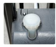
Brake fluid reservoir with level switch
