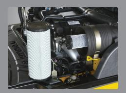
**Quick-change air cleaner**The 6-inch cyclone air filter is readily accessible for cleaning or replacement.
