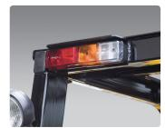
Rear safety lamp Rear combination lamps with directional indicators, rear lights and brake lights are positioned to provide a higher level of safety.
